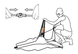
With the hub in an upright position, unfold the poles and lock the joints.
