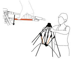
Using your thumbs, push the orange poles downwards to disengage the hub and collapse the shader.
