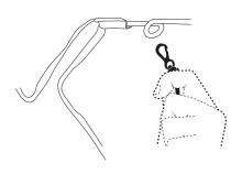
Hang the spring clip of the cord on the hanging loop located at the edge of the canopy ribs.
