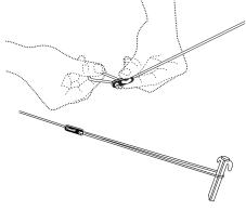
Adjust the cord length using the runner. Tense the cord by anchoring it to the ground with the peg.
