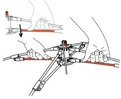
Standing behind the shader, grab the left and right poles. Using your thumbs, push the orange poles downwards to collapse the shader.
