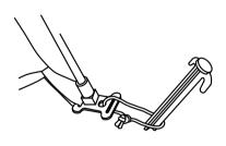
Lock the hub by turning the orange button found on the hub, to the "LOCK" position.
